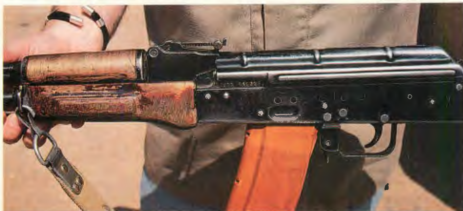
TOP: Brown found AK-74 exceptionally easy to control in full-auto mode due to muzzle brake. ABOVE: AK-74, held by Brown, is little different from AK-47 except for caliber, extractor and muzzle brake.
